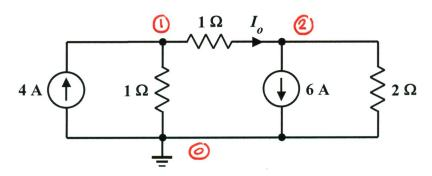
a. How many equations are necessary to analyze this circuit by the nodal analysis method?
